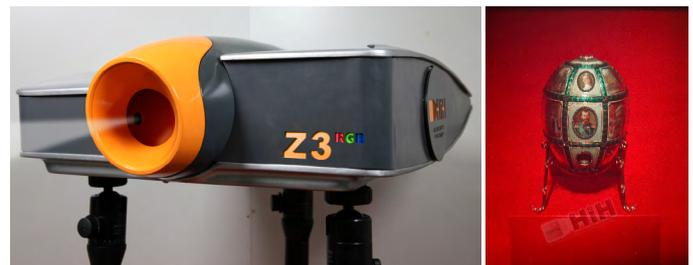
Figure 2: (L) An example of a portable holographic system called ZZZyclops developed at Hellenic Institute of Holography in Greece and (R) an example of a hologram written with the ZZZyclops.
