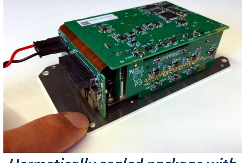
Hermetically sealed package with integrated electronics
