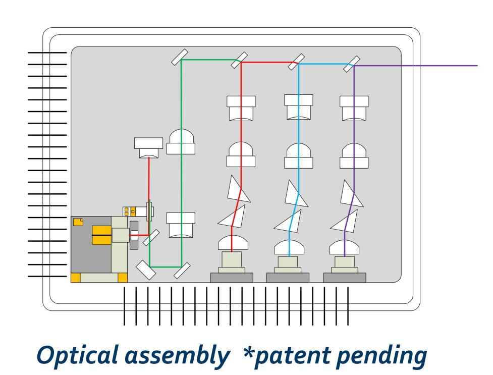
The HTCure<sup>m</sup> laser manufacturing technology allows for a high precision mounting and ultra-stable permanent alignment of the output beams. A novel production process (*patent pending*) enables a beam overlap of better than 150 µrad. The optical platform can be customized for a higher degree of integration into the flow cytometer.
